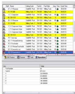
Fig. 6. Pocket milling using “concentric out” strategy.
