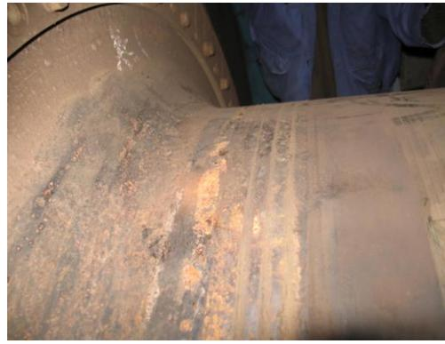
**Fig. 3.** Corrosion disposed on circumference (HA 8).
