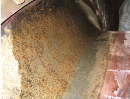
**Fig. 2.** Spot corrosion (HA 1).
