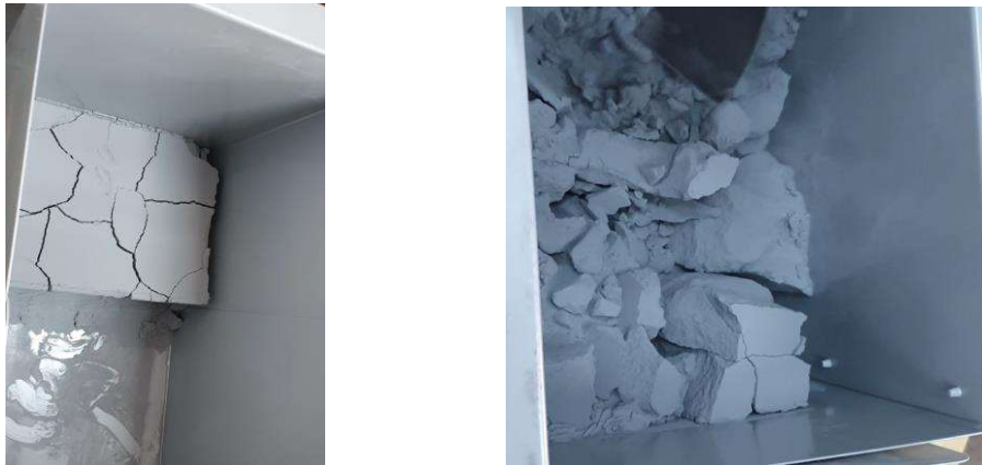
Fig. 6. Post-processing parts printed with SLS technology.
