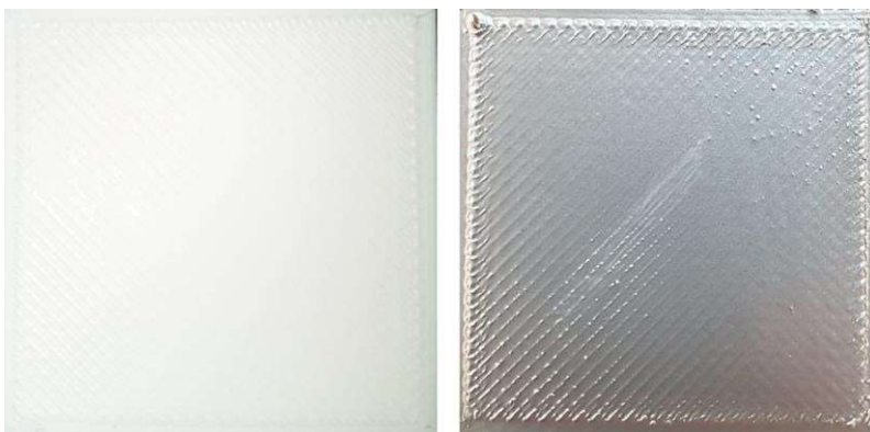
Fig. 12. 3D printed ABS white color part before and after painting process with chrome spray.
