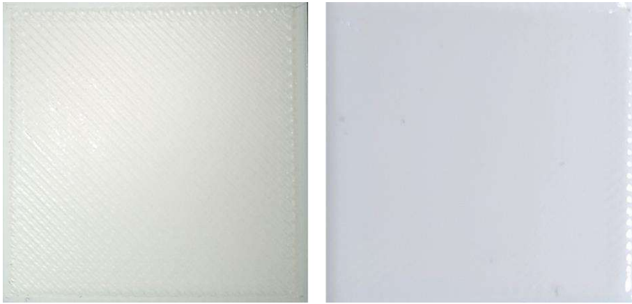
Fig. 10. 3D printed ABS-white color surface part before and after post-processing with industrial Acetone [16].
