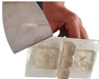
Fig. 4. Removing the parts from the building platform with the help of a putty knife.
