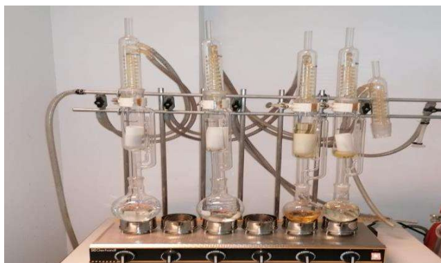
Fig. 2. The SOXHLET extraction system (Laboratory for Analysis, Control and Remediation of Contaminated Soils/CAMPUS)
