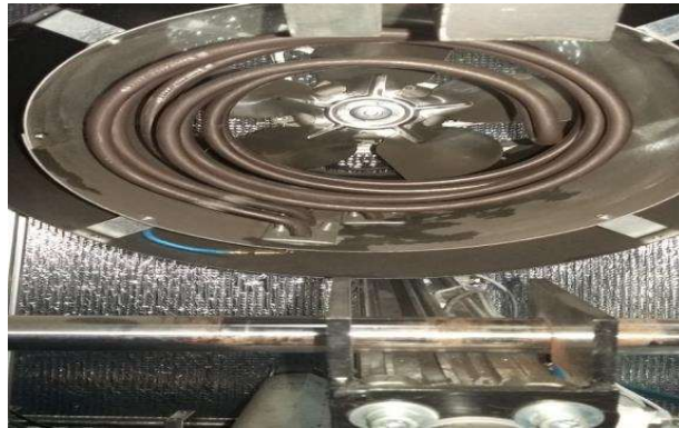
Fig. 3. Fan to provide control of temperature on the equipment enclosure
