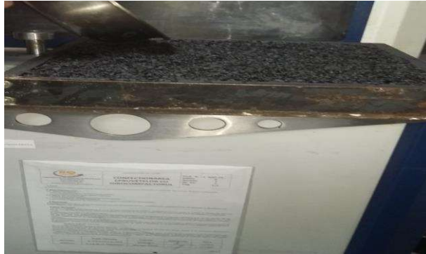
Fig 5. The plate with asphalt mixture and the product CARGOSFSLT UV (THERM)+anrobrate aggregates
