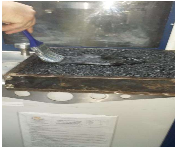
Fig 4. Preparing the plate with the asphalt mixture + CARGOSFALT UV (THERM) product
