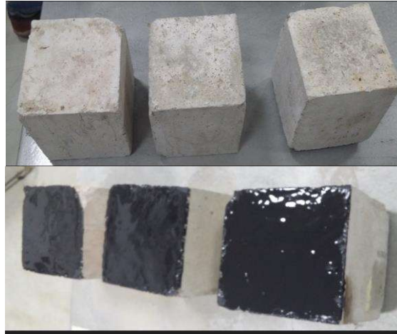
Fig 8. Reference concrete cubes and treated concrete cubes with CARGOSFALT
