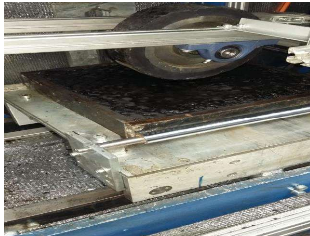
Fig 6. Roller sled of the wheel tracking test equipment
