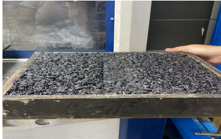
Fig 3. The asphalt mixture after the wheel tracking test at 70°C
