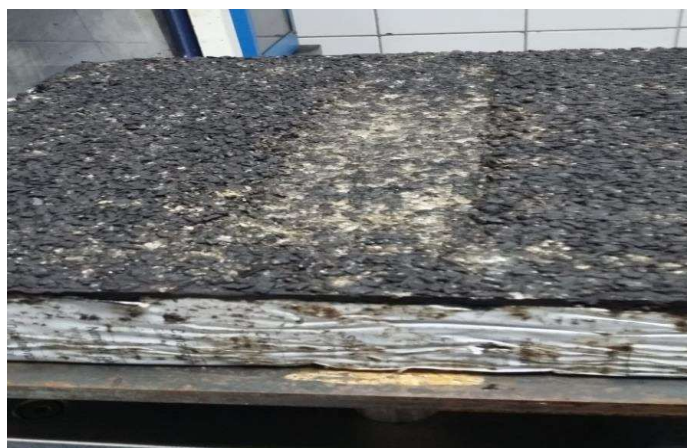
Fig 7. Footprint on the plate with asphalt mixture and the product CARGOSFALT UV (THERM)
