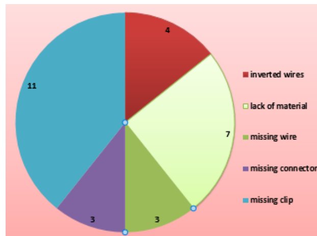
Fig. 4. Number and type of internal defects registered in January 2020
