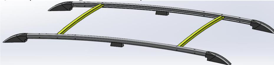
b). Examples of mounting L2 bars in active position folded down at minimum distance
