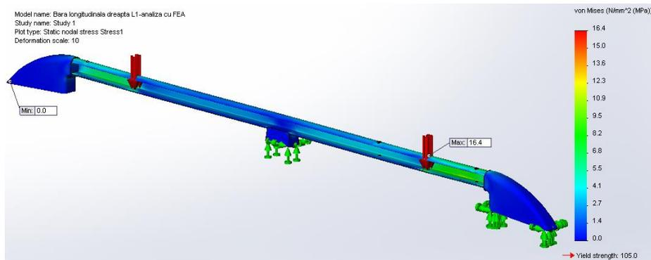
**Fig. 11** The state of vonMises equivalent stress, [MPa]
