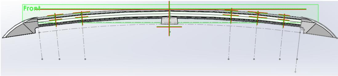
a) Sketch of the longitudinal and flat bar used in the construction of the 3D model in the version with holes (for joints and fastening / folding) in normal position (radial);
