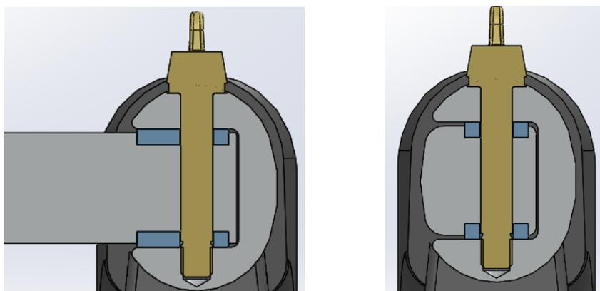
a. L1 bar. Sections in one of the three attachment points of the free end of the T1 bar with butterfly head screw for mounting/ folding positions
