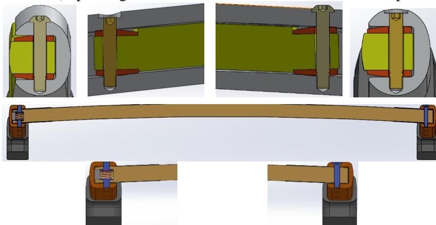
**Fig.6** Details of longitudinal and transverse sections in the L3 bar in the rows with holes (for joints and fastening/folding) and various types of joints inclusive rapide joints
