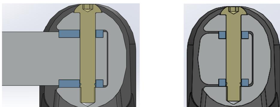
b. L1 bar. Sections in one of the three attachment points of the free end of the T1 bar with screw with semirotund head and hehagonal locas for mounting / folding positions
