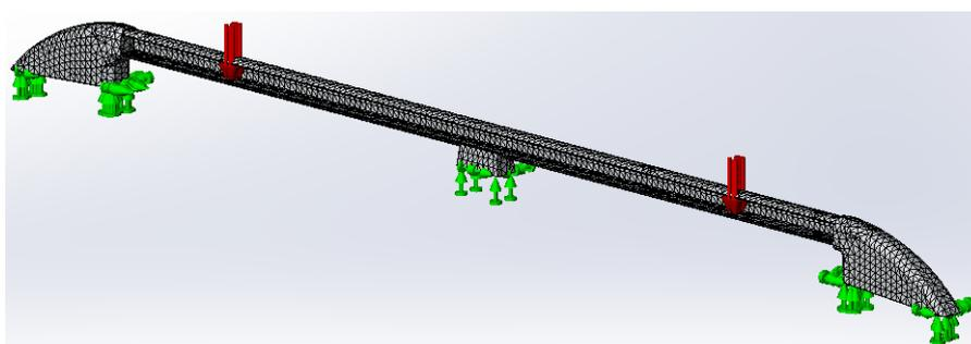
Fig. 10 Diagram of calculating the L1 bar, constant section and rectangular recess
