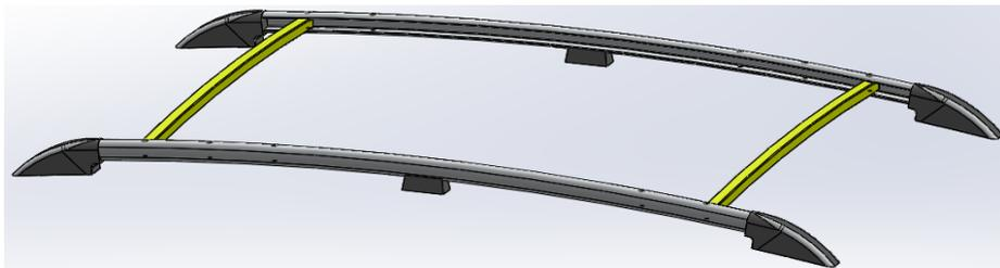
a). Examples of mounting L2 bars in active position folded down at maximum distance
