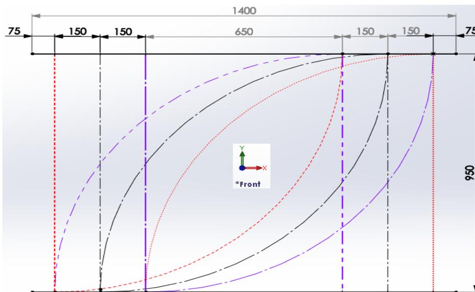
**Fig. 7.** The geometrical places described by the ends of the folding crossbars, when moving them from the folded poz to the extended position
