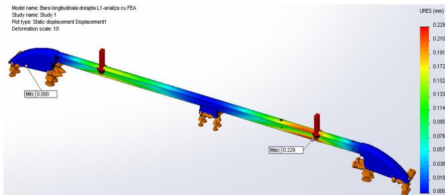
**Fig. 12** Field of the resulting deformations [mm]
