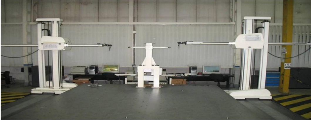
Fig. 5 3D measuring machine – for stamped parts
