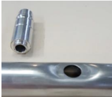
Fig. 3. The tube before welding
