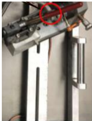
Fig. 8. Identification of the leakage point
