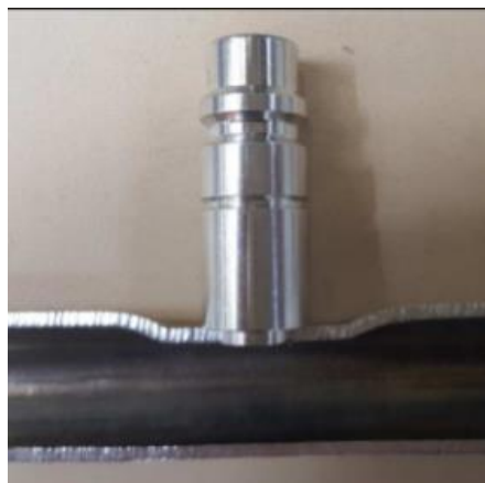
Fig. 4. The tube after welding
