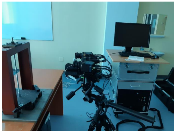
Fig. 9. Aragement for GOM stereo-camera and acquisition system
