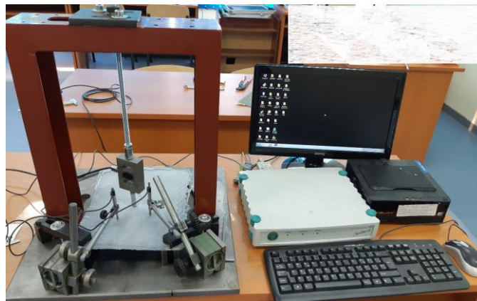
Fig. 8. Aragement for force and travel transducer and the acquisition system
