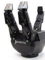
Fig. 2. Three finger adaptive gripper ( http://robotiq.com/products )
