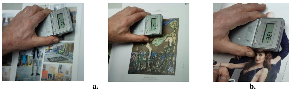
Fig. 10. Optical density measurement with a densitometer a. brochure "Saloanele Moldovei"; b. magazine "Formula krasoti"
