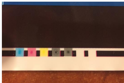
Fig. 12. The size of the 1 mm point formed at the intersection of the rays built in squares, indicate the correct pressure at the associated inking unit.
