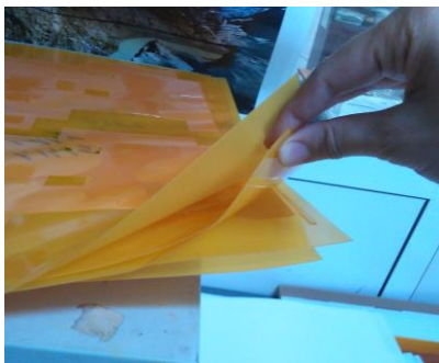
Fig. 5. Set of printing plates for only one product.
