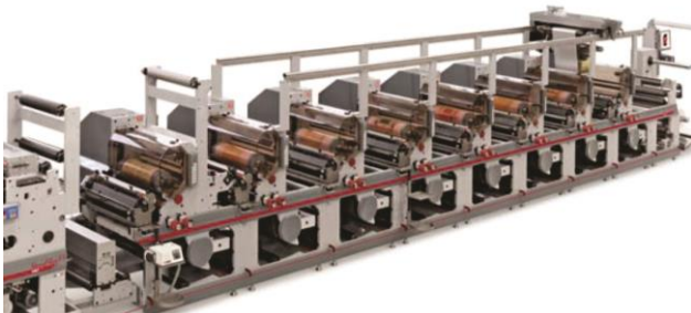
Fig. 3. Printing assembly of the flexographic machine.
