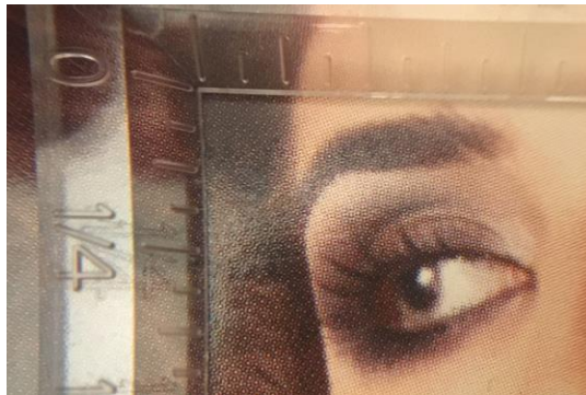
Fig. 13. The verification with the typographic magnifier is the usual method for permanently controlling the impression on the printing flow.
