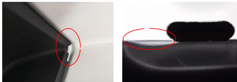
Fig. 1. Quality defects caused by inappropriate covering.
