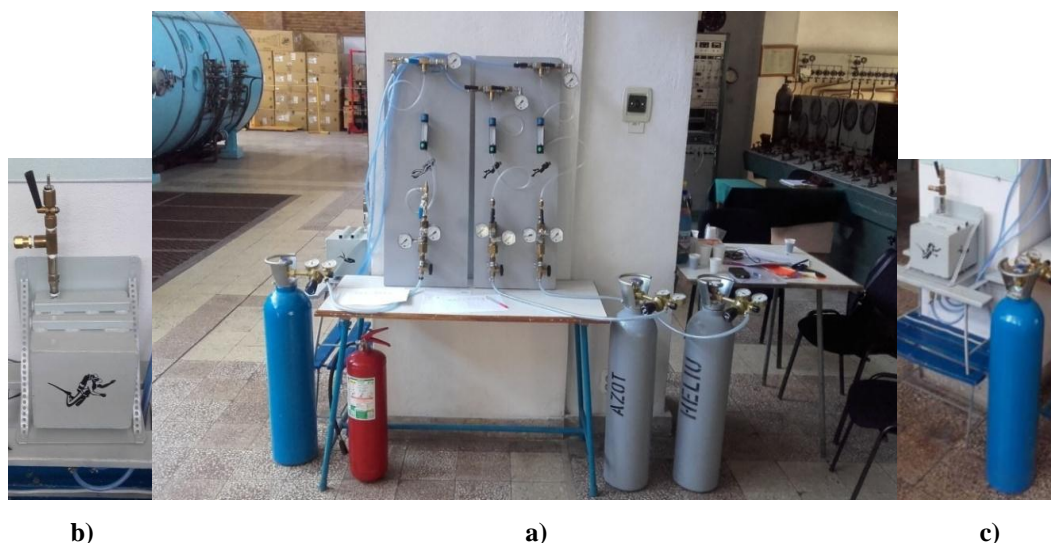
Fig. 2. - The Experimental Installation for Preparation, in Continuous Flow, of the Breathable Gaseous Mixtures – a) and the Mixing Chamber – b), c).
