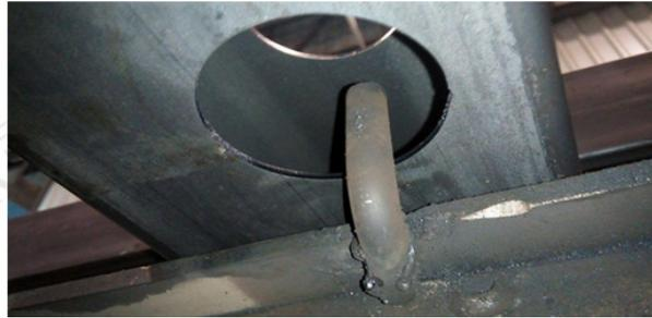
Fig. 8. Interdiction Poka-Yoke device.
