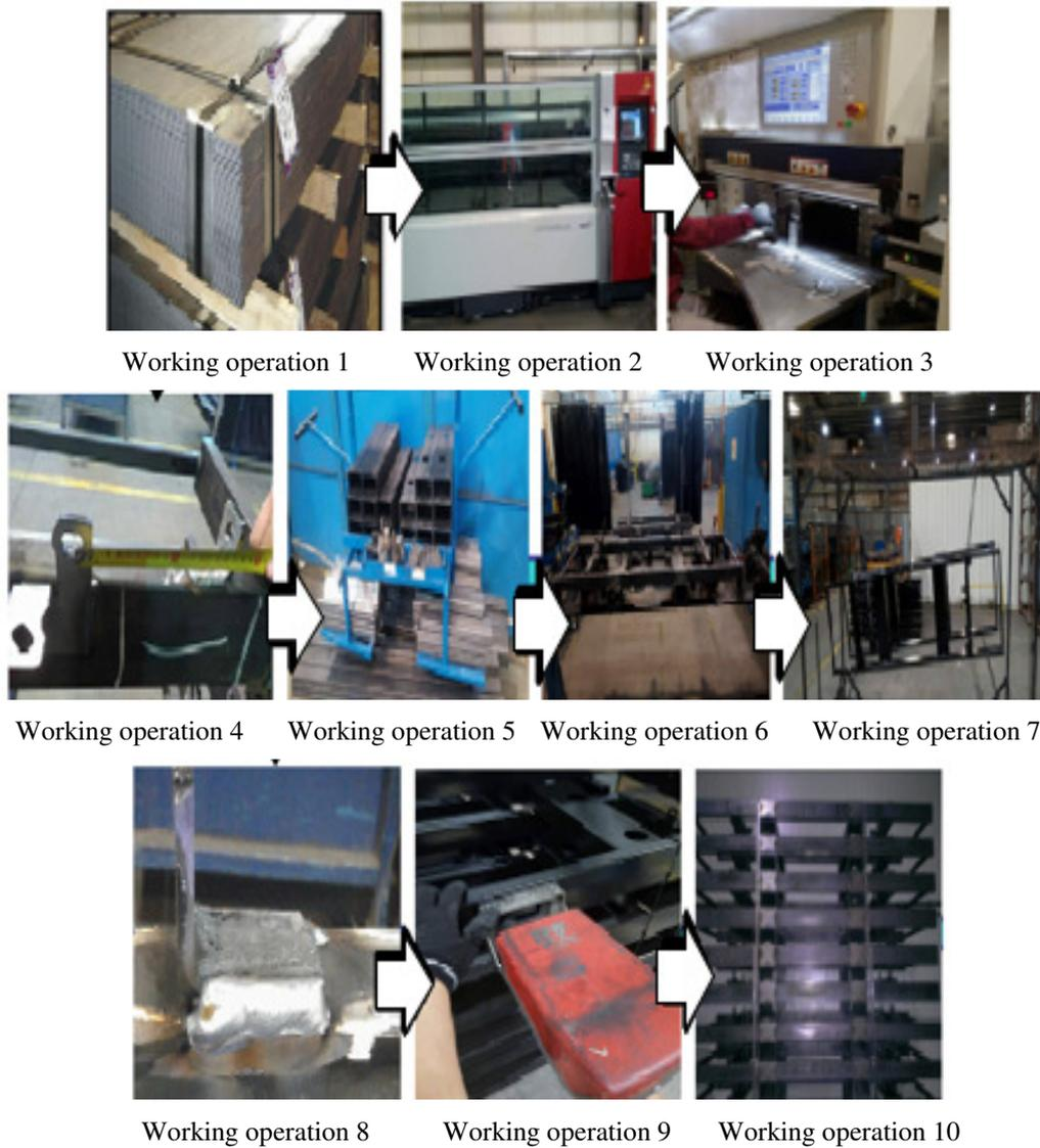
**Fig. 4.** The stages of the technological process of “pallet for transport”.
