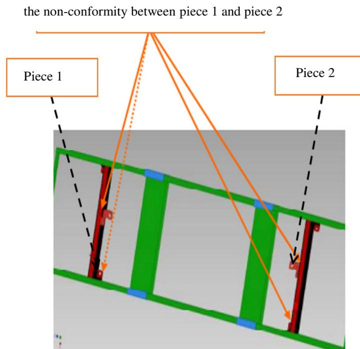
**Fig. 5.** The type of defect identified on the product „pallet for transport”.
