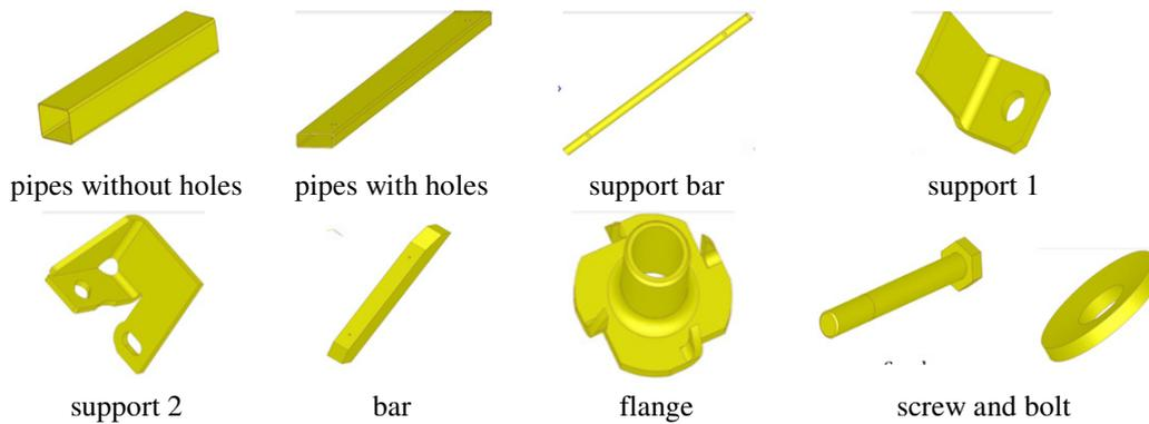
**Fig. 3.** The components of the “pallet for transport”.
