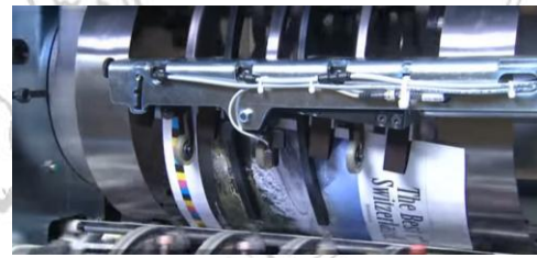
Change over from gripper to suction opening.
