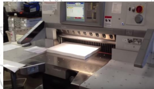
Cover cutting to the gross format [7].
