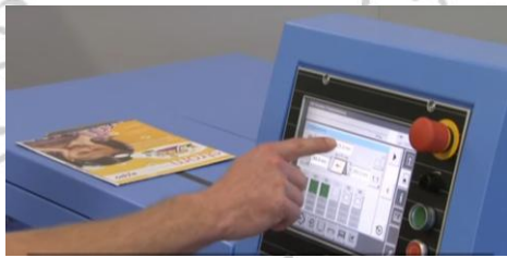
Programming the automatic line functions from the processor console.
