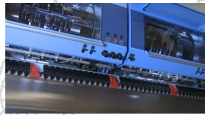
Automatic synchronization of feeding stations.
