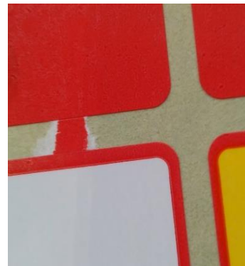
Fig. 5. Incompletely cut labels that remain attached.
