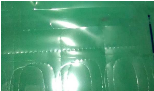
Fig. 14. The die cut print generated by perfectly paired die cuts executed independently. The shift in the drawing of the die cut nests is noticeable.
