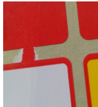
Fig. 5. Incompletely cut labels that remain attached.
