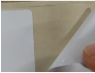
Fig. 11. The die does not correctly cut the face of material.
