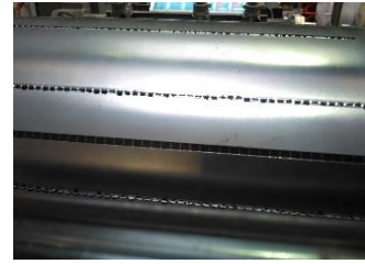
Fig. 13. Destroyed die in the perforation area. It is mounted on the magnetic cylinder
