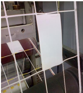
Fig. 3. The label remains trapped in the waste matrix.
