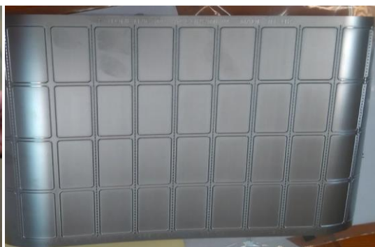
Fig. 2. A flexible die. Its front face is the part with shapes defined by the cutting blades.
