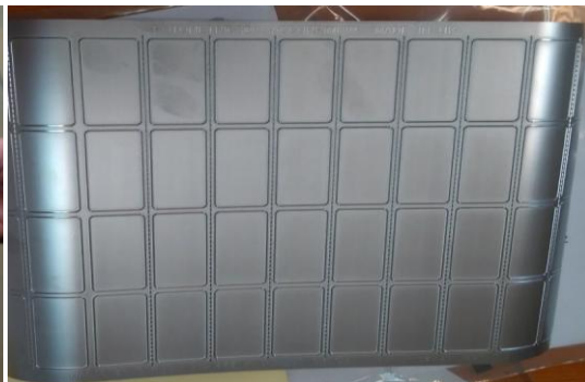
Fig. 2. A flexible die. Its front face is the part with shapes defined by the cutting blades.
