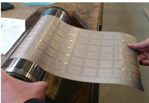
Fig. 1. The die is flat-shaped. It is mounted on the magnetic cylinder by rolling.
