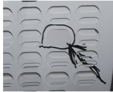
Fig. 8. Waste not removed by die cutting. The product is nonconform.
