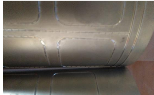
Fig. 15. Matching die cuts independently executed. Checking the nest overlap is done by matching the die cuts at the edge.
