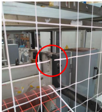
Fig. 4. The waste matrix is broken.
