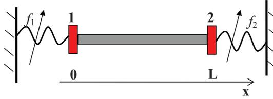
Figure 2: Two Van der Pol oscillators on the elastic rod
