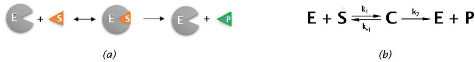
Figure 1: The schematic (a) and the symbolic (b) representations for the Michaelis-Menten mechanism
