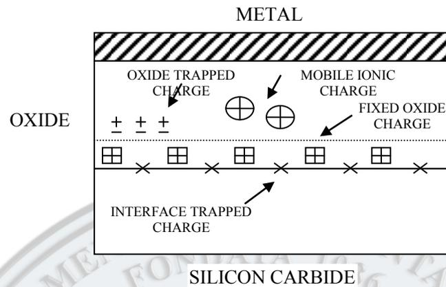
Fig. 2. Oxide trapped charges in MOS structure.
