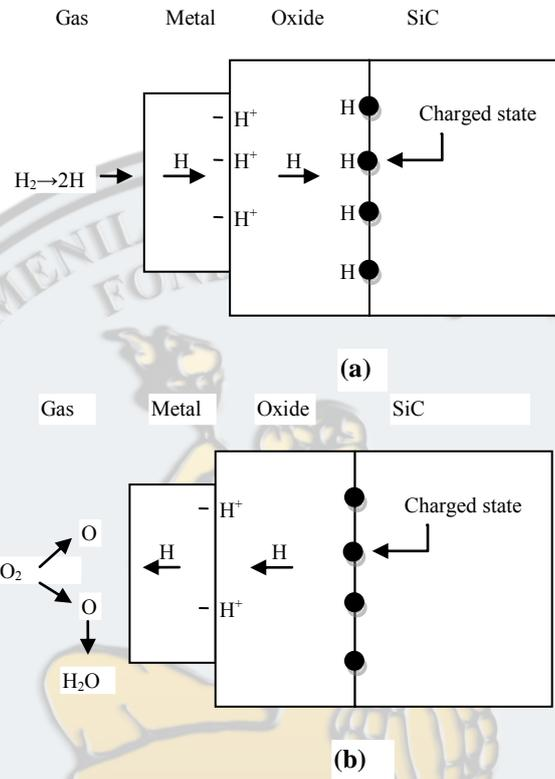
**Fig. 7.** Charge distribution in: (a) hydrogen, (b) hydrogen and oxygen exposed MOS capacitor gas sensor.
