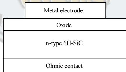
**Fig. 4.** SiC MOS capacitor hydrogen sensor structure.
