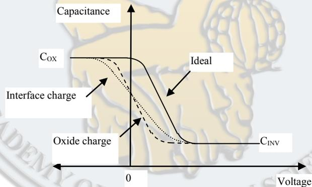
Fig. 3. Comparison of C-V characteristics of ideal and real MOS capacitor.
