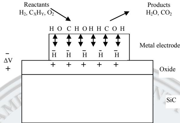
**Fig. 5.** Sensing mechanism for MOS capacitor hydrogen sensor.
