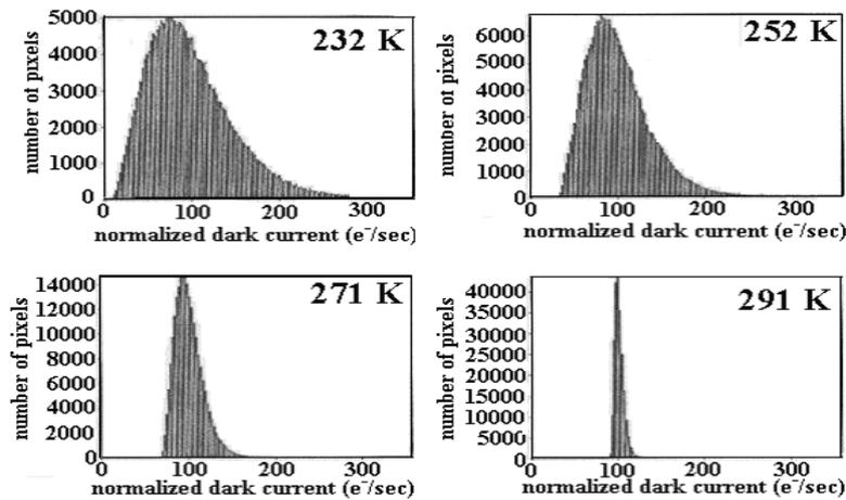
Fig. 1. Dark current normalized to 100 e<sup>-</sup>/s [9]
