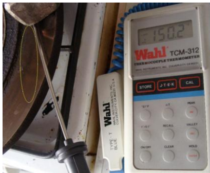
Fig. 14 Temperature indicated by contact thermometer (150.2 °C) and selected area for histograms.
