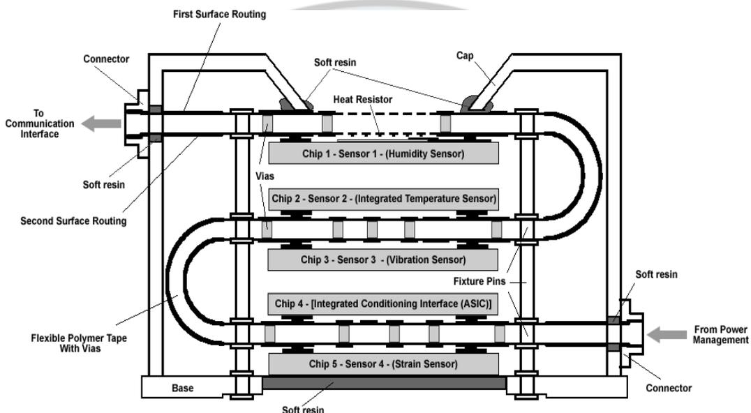
**Fig. 6.** Folding the tape for getting a 3D stack.
