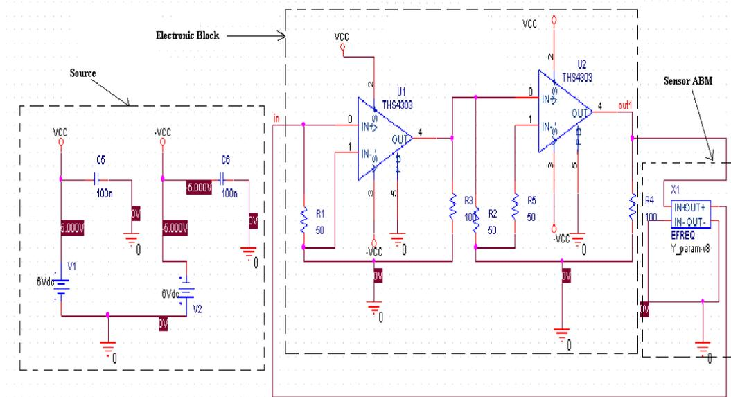
Fig. 10 (a). Electronic schematic of an oscillator with the SAW sensor in the feed-back loop.
