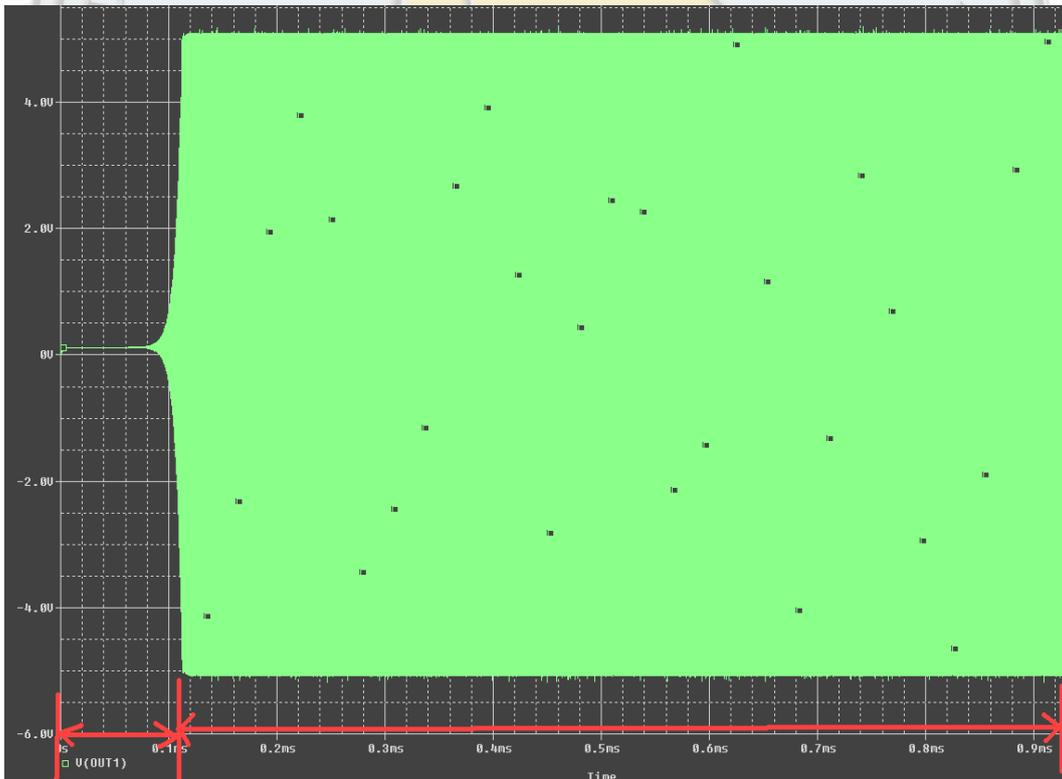
Fig. 10 (b). Start transient regime and steady state of the oscillation.
