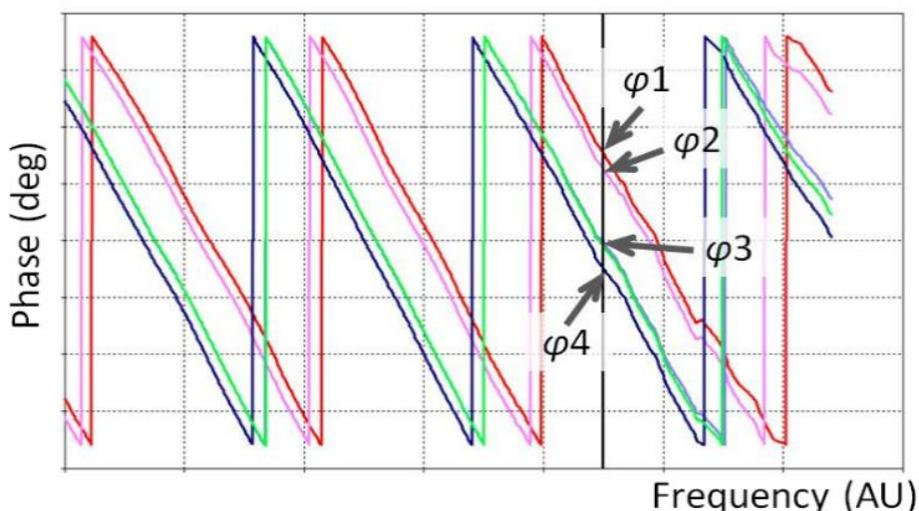
**Fig. 4.** Phase changes due to variable concentration of the specific analyte.
