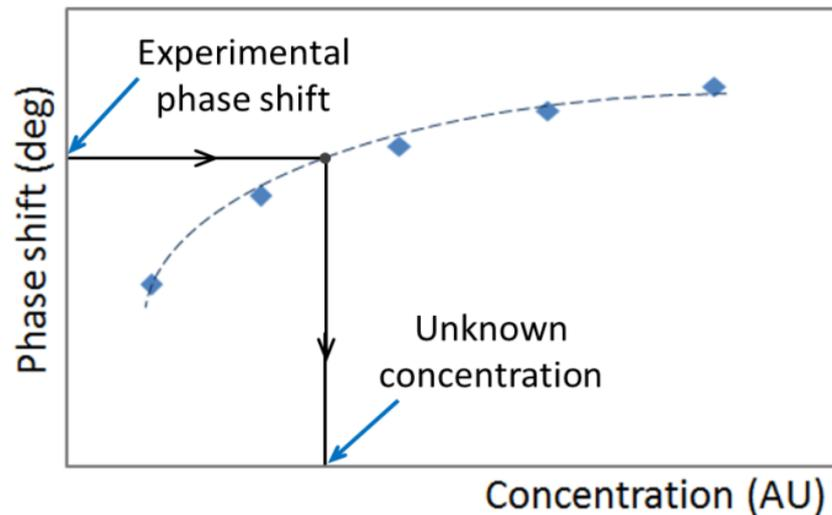
**Fig. 5.** Example of calibration graph based on experimental results.
