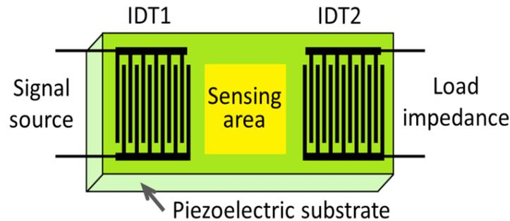
**Fig. 1.** Structure of a transmission type SAW sensor.
