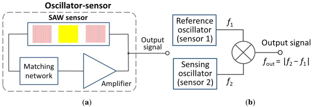
**Fig. 6.** Block diagram with single oscillator incorporating the SAW sensor measurement cell (a), and differential, dual oscillator structure (b).
