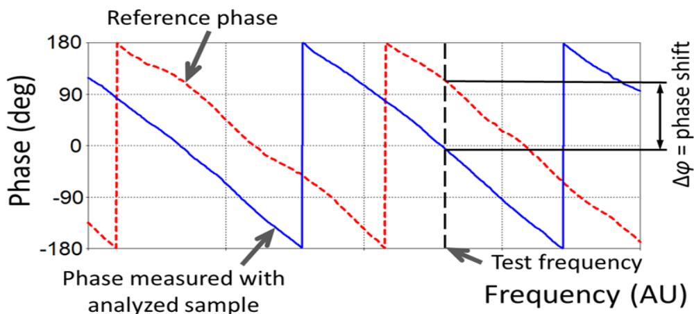
**Fig. 3.** Phase shift  $\Delta\varphi$  of the transmission parameter observed as phase difference between empty cell (reference value) and in presence of the analyte.
