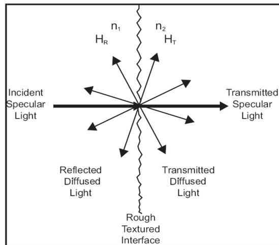
**Fig. 2.** Relationship between the haze functions and the specular and diffused light at a textured interface.
