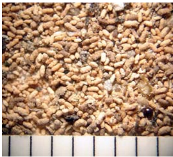
Fig.14 - Aspect of sawdust caused in the beech tree wood by th species Anobium punctatum (original)
