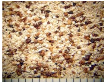
Fig. 18 - galleries and sawdust from fir tree wood caused by the species Ernobius mollis (original)
