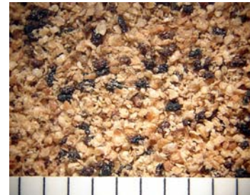
Fig. 19 - aspects of the sawdust caused by the activity of species Hylotrupes bajulus in th fir tree wood (original)
