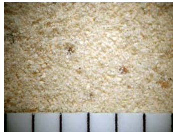
Fig. 15 - Aspect of sawdust caused by species Lyctus linearis in the elm tree wood (original)
